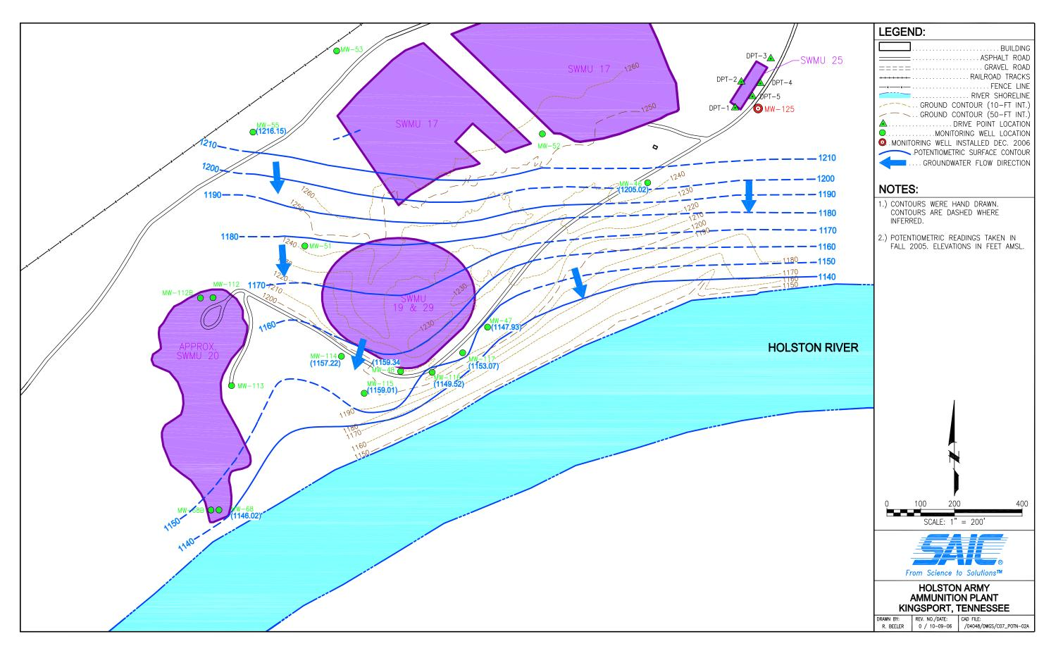
Figure 2. Groundwater Potentiometric Surface at SWMUs 19 and 29, Fall 2005
