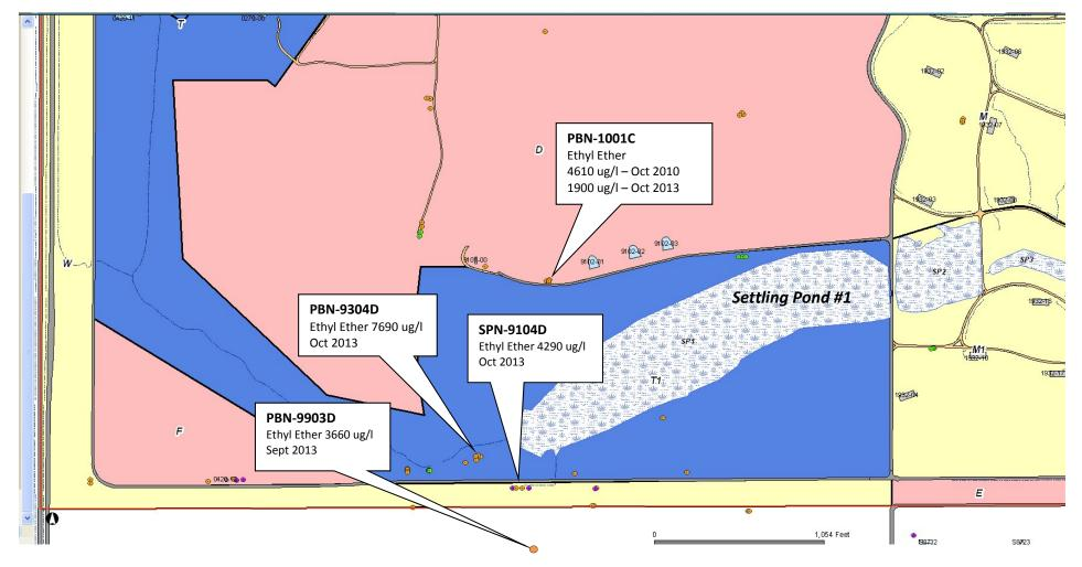
Southwest Corner of Badger Army Ammunition Plant. Groundwater monitoring well PBN-9903D is outside the plant boundary. The Wisconsin NR 140 Public Health Enforcement Standard for ethyl ether is 1,000 ug/l.
