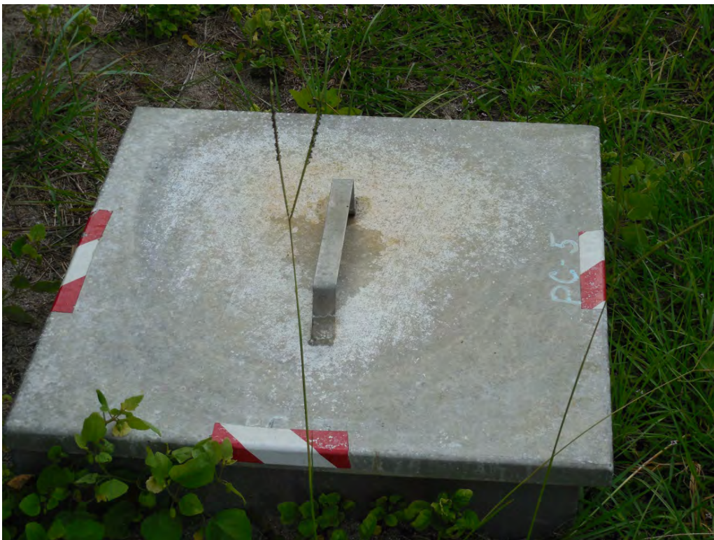
Photo 16: Typical fabricated monitoring well protective cover.
