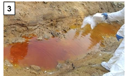
... to turn bright red: oxidation is underway Time: 10 secs after application
