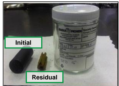
33g of NC propellant reduced to <5g of non-explosive residual in less than 48 hours
