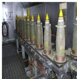
Preparation of projectiles for waterjet cutting and washout in Gradient's booth
