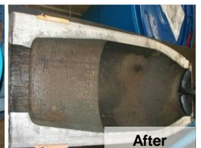
Rapid decontamination of halved bomb casings before and after MuniRem® treatment
