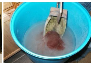
Rapid decontamination of halved bomb casings before and after MuniRem® treatment
