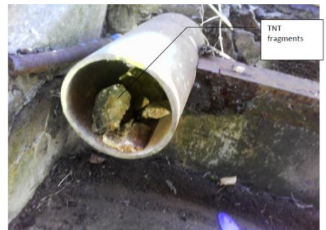
The 150 mm pipe (discharge end) before set up
