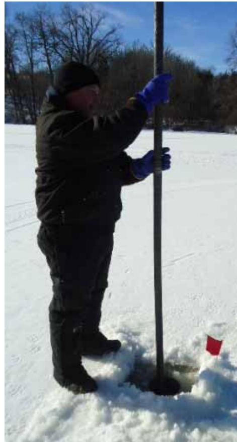
Lowering WDNR probe to measure bottom of the sediment
