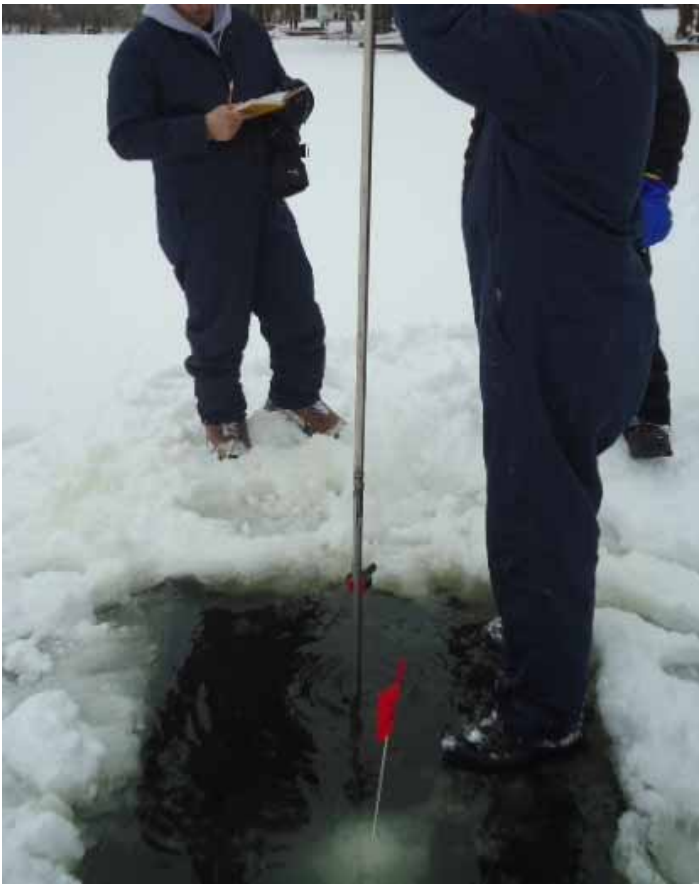
Driving SPS probe to measure bottom of the sediment
