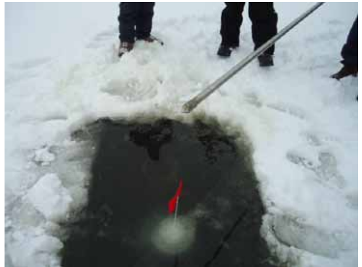
SPS probe for measuring the bottom of the sediment
