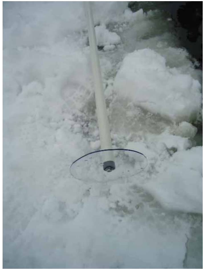
Probe for measuring the top of the sediment
