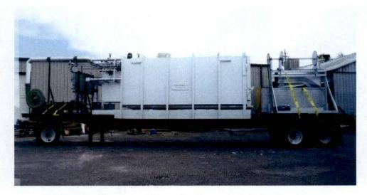
FIGURE 2: All components are stored on a single trailer for shipping
