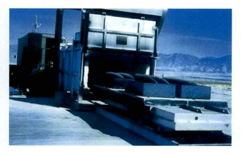
FIGURE 1: The US Army developed a simple flashing furnace with a rolling hearth (seen processing 750 lb. bomb shells)
