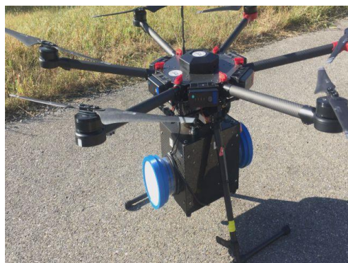
Figure 2-3. UAV-Based Sampling Method
