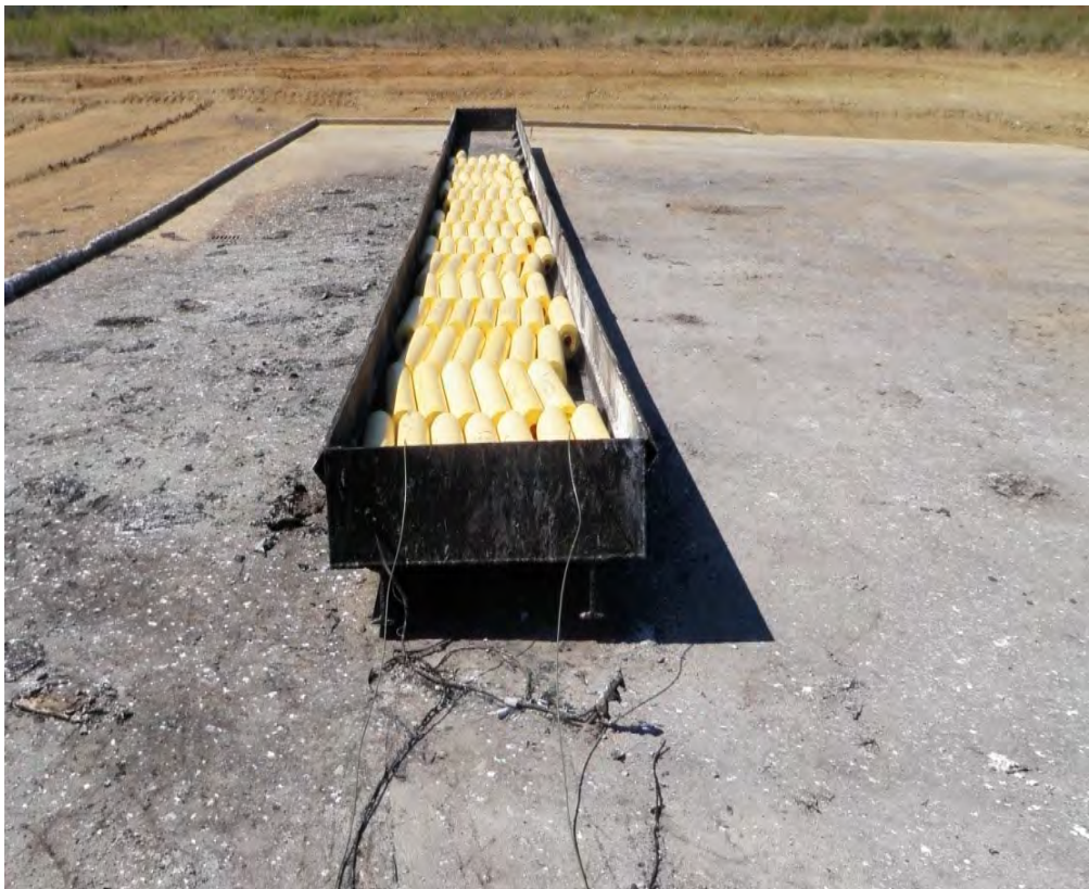
Photo 2: OB Unit – Looking West - Propellant Charges in Concrete Pad with Time Fuze
