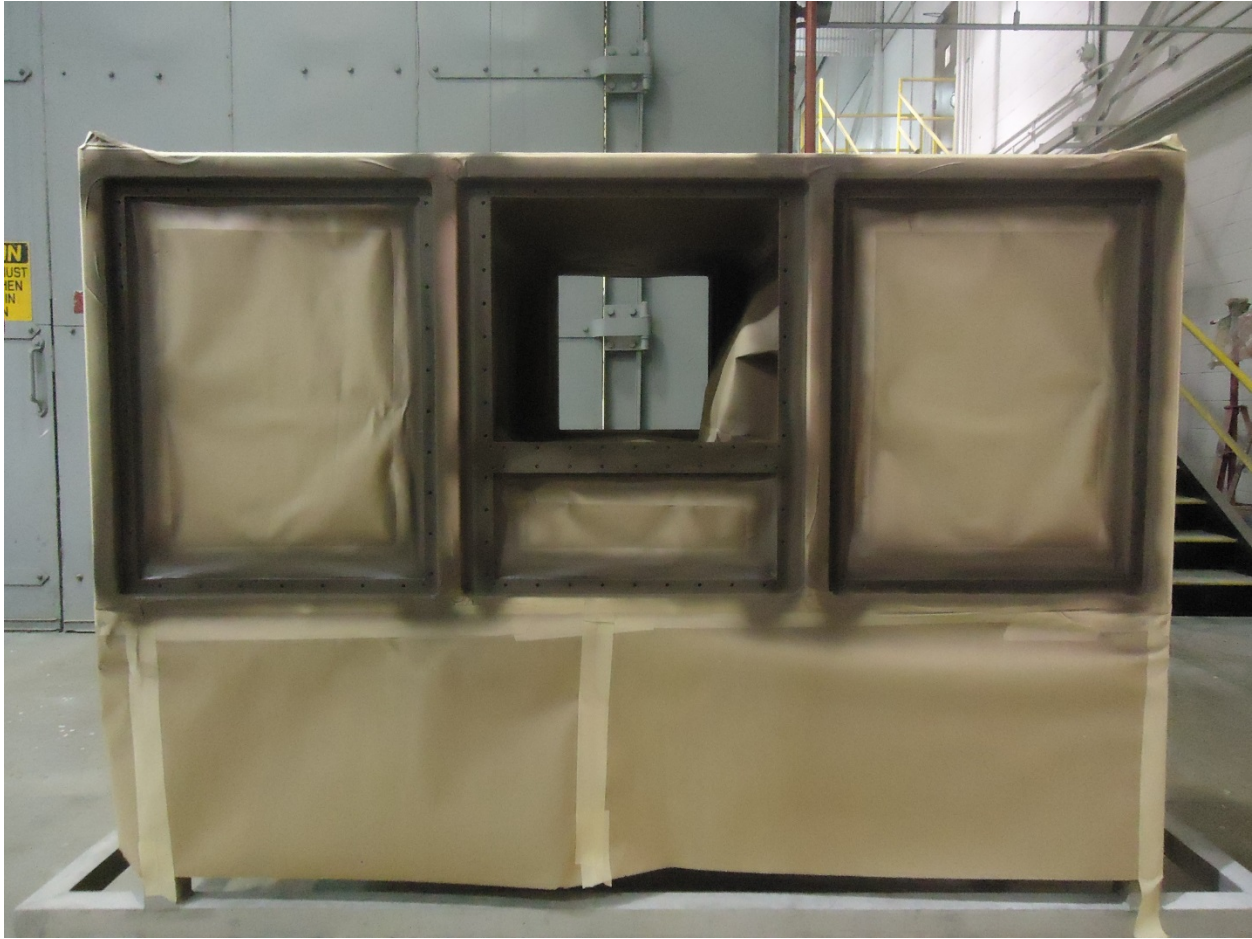
Figure 7. Cho Shield 2003 Applied to Electronics Cabinet
