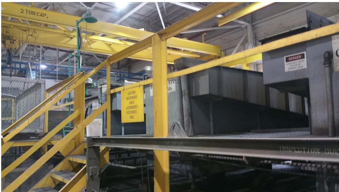
Figure 5. Chromate Conversion Coating Tanks in LEAD Building 350
