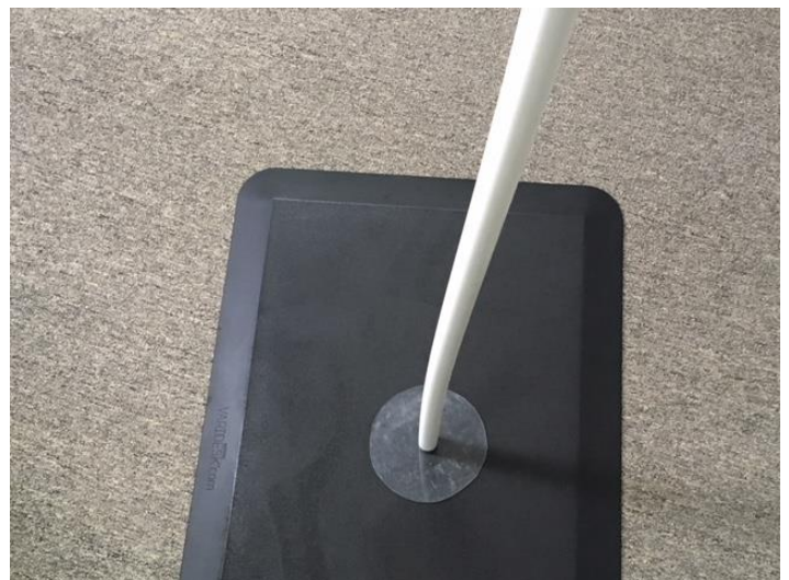
Probe for measuring the top of the sediment
