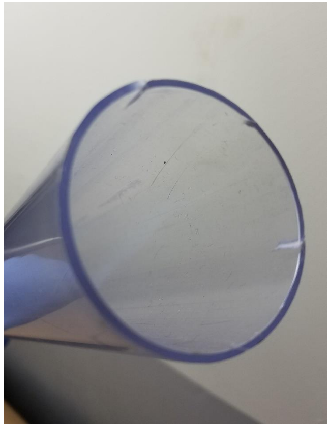
2-inch diameter semi-clear plastic disposable liner
