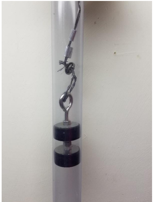
Inner dual piston within the plastic liner
