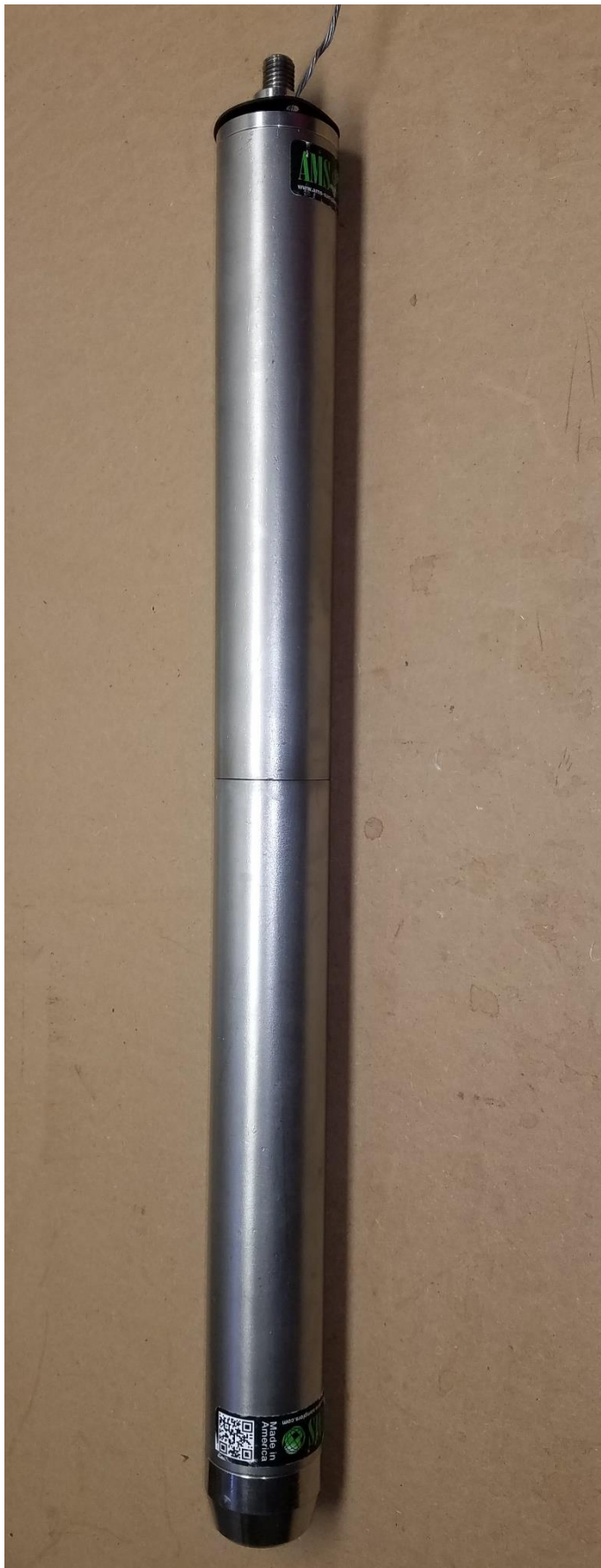
AMS multi-stage sediment sampler - 2-foot section
