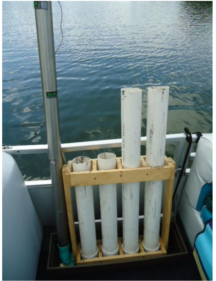
Storage system to keep samplers vertical during transport to field trailer
