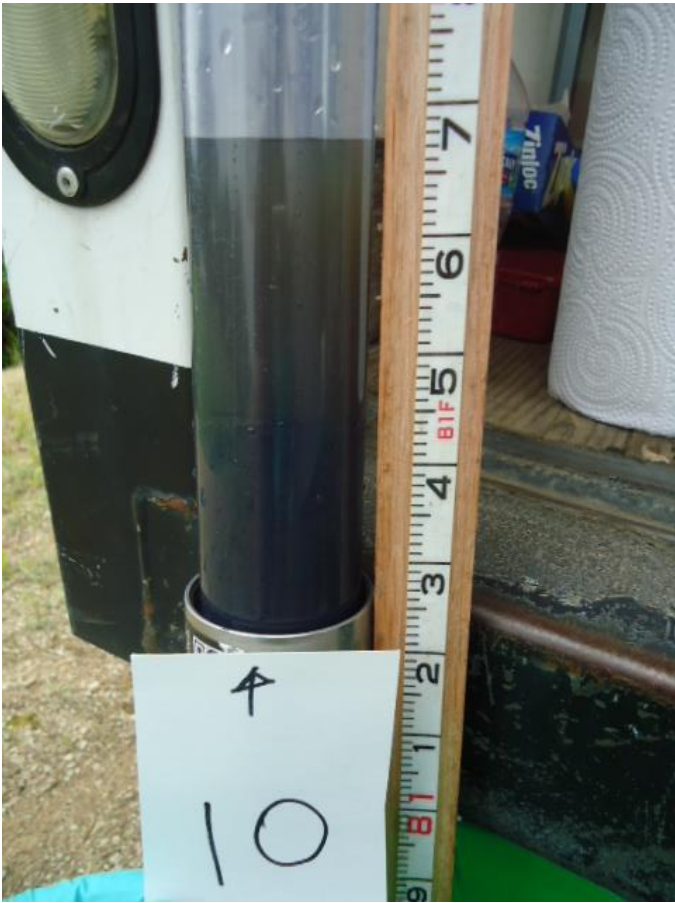
Plastic liner displaying sediment sample and retained water
