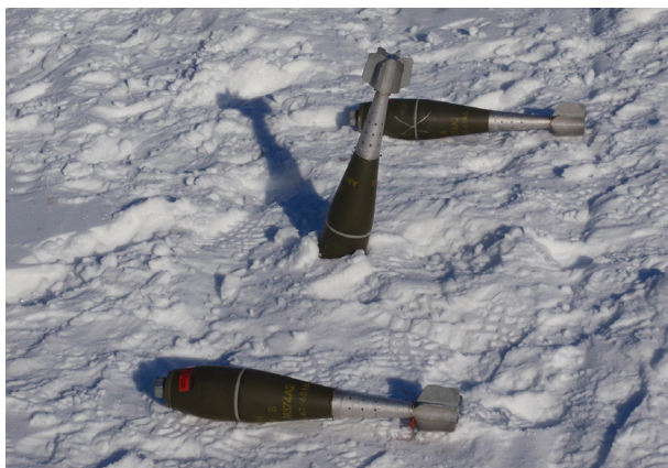
FIG. 3: Close-proximity detonation test setup. The center round will detonate, simulating a functioning round. Horizontal rounds simulate unexploded ordnance.
