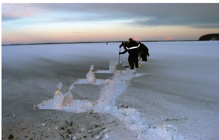
FIG. 1: Discrete samples being taken from a highly loaded segment of a detonation plume
