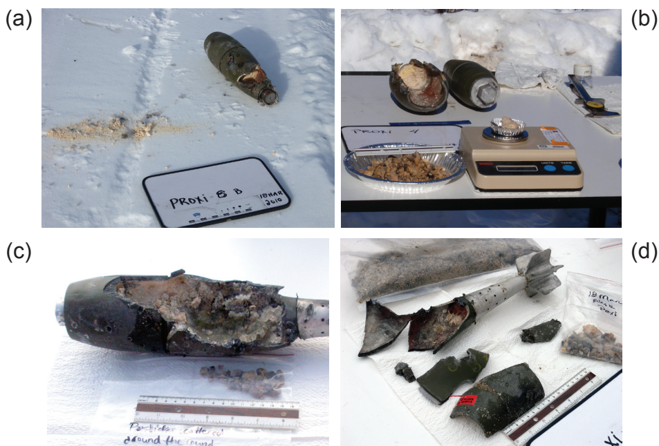
FIG. 4: Damage to surrogate UXO from close-proximity detonations. (a) Pierced (breached) round. (b) Partial detonation (left) with most of filler ejected. (c) Partial detonation with most of filler intact. (d) Low-order detonation with larger body pieces.
