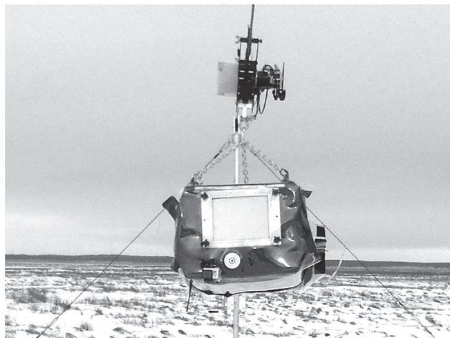
Fig. 2. Flyer airborne sampling instrument.
