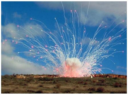
Figure 1. Open Detonation Showing Uncontrolled Emissions and Kickout
