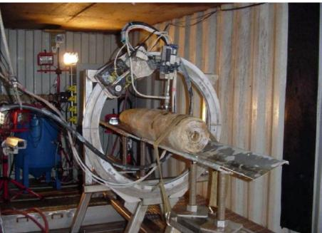
**Figure 5. Fluid Jet Cutting**
