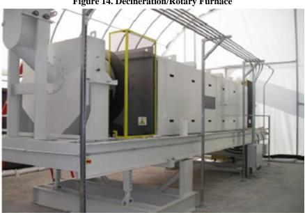
Figure 14. Decineration/Rotary Furnace
