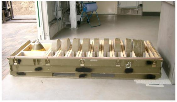
Figure 6. Segments of Bomb Cut by Underwater Band Saw
