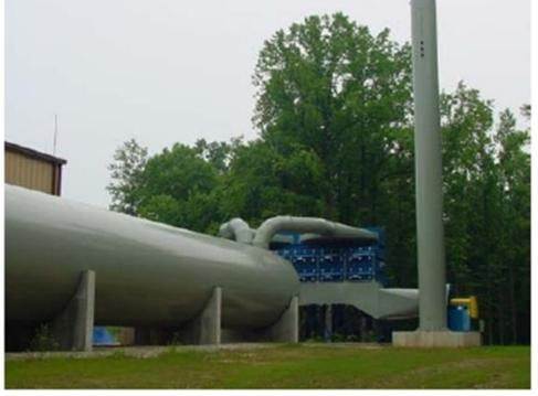
**Figure 9. Controlled Detonation Chamber**
