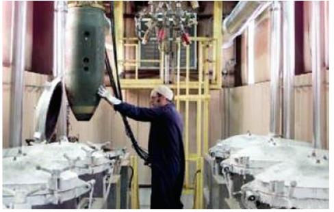
Figure 7. Autoclave Meltout
