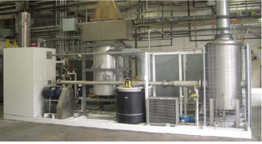
Figure 13. Industrial Supercritical Water Oxidation
