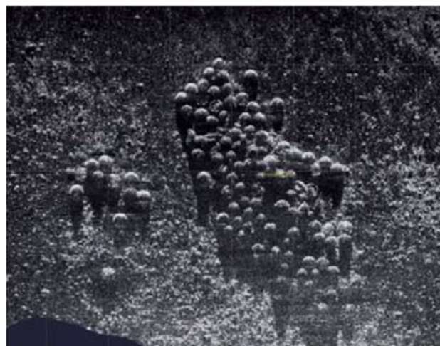
Fig. 2 Hi-SAS-Sonar image of some 70 moored mines from the Second World War in study sub-site 1 in the Kolberger Heide. Source: Deutsche Marine 2012
