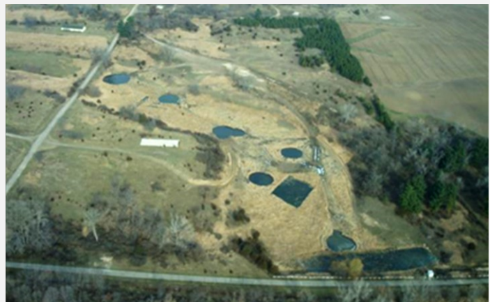
The Army excavated "hot spots" (shown here in this 2009 photo) to remove soils with the highest contaminant levels at the Settling Ponds. At the time, mercury was not identified as a contaminant of concern. However, recent testing has detected elevated levels in the soil.
