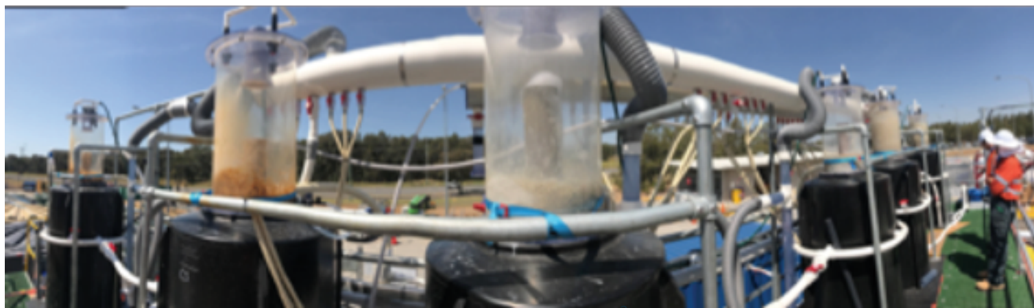
Figure 1 Ozofractionation used to treat more than 15,000 m 3 of PFAS-impacted wastewater
