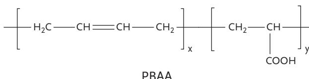
**Figure 1.3** Chemical structure of PBAA.
