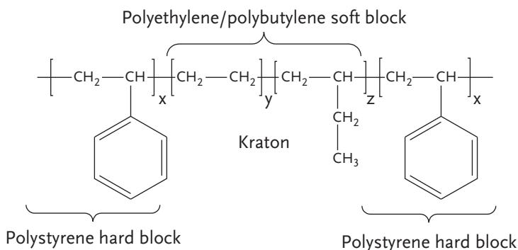
**Figure 1.10** Chemical structure of Kraton.
