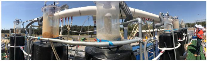
Figure 5. Ozofractionation system in action to remediate PFASs in a C6 fluorotelomer foam spill in Brisbane, Australia. Source: Ian Ross, Arcadis/ EVOCRA.
