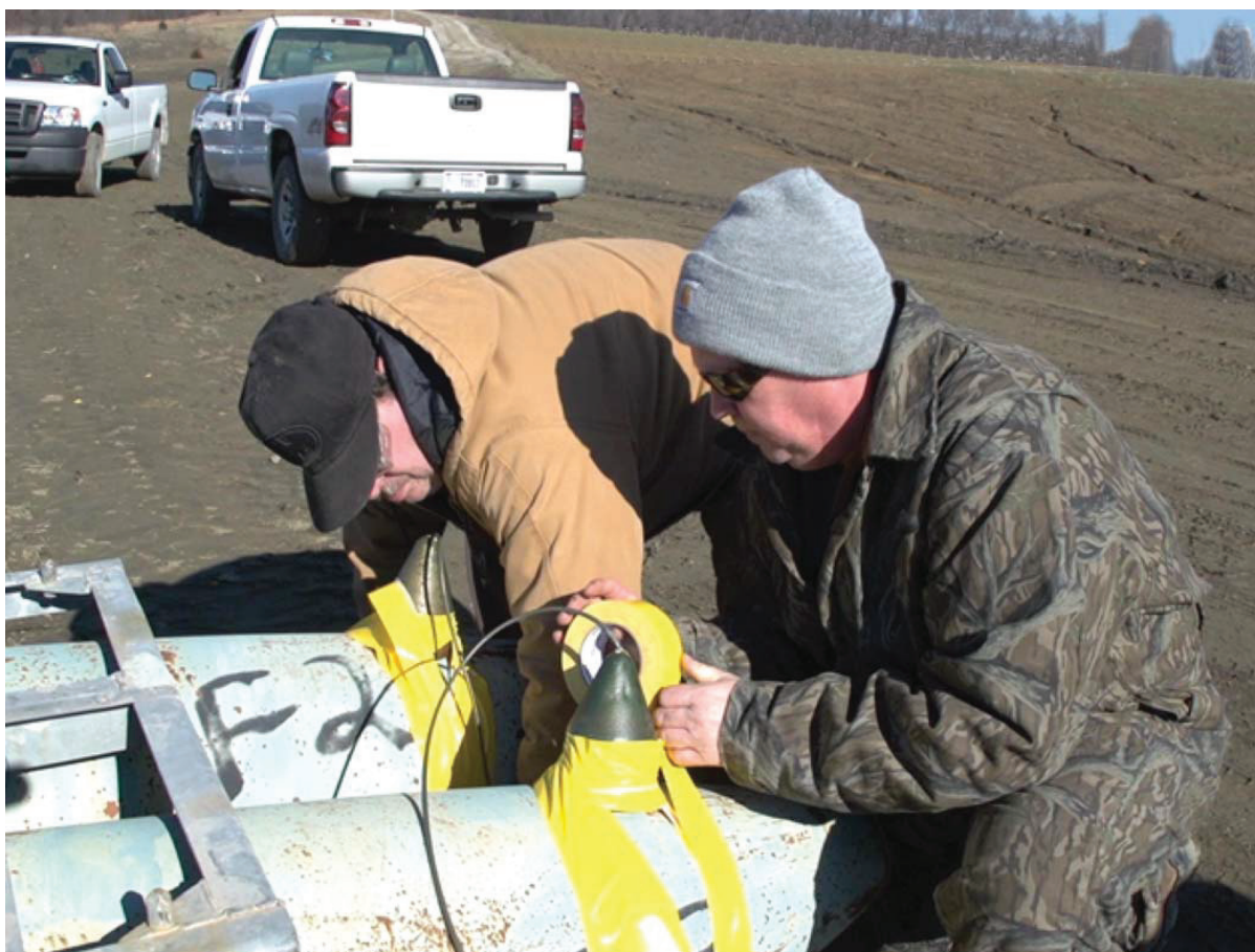
FIGURE 3.5 Technicians prepare bombs for venting (a form of OD) at the Crane Army Ammunition Activity. SOURCE: Joint Munitions Command Public Affairs Office.
