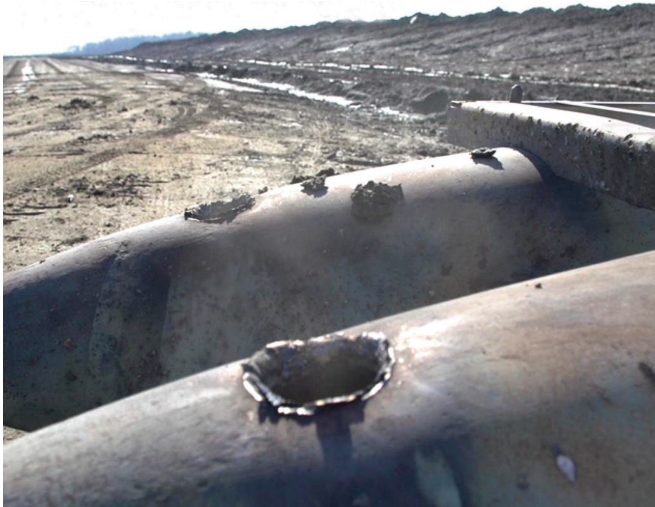
FIGURE 3.6 Vented bombs at Crane Army Ammunition Activity. SOURCE: Joint Munitions Command Public Affairs Office.
