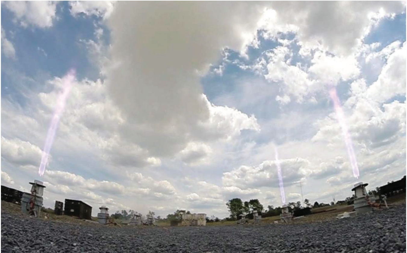
FIGURE 3.3 Static firing (a form of OB) of Shrike rocket motors at Letterkenny Munitions Center. SOURCE: Joint Munitions Command Public Affairs Office.
