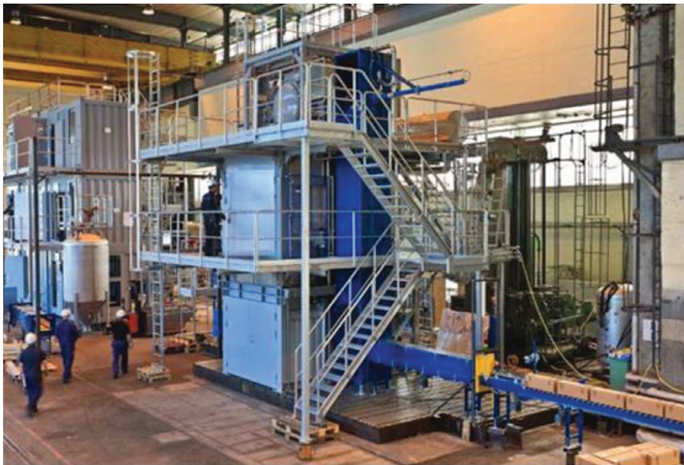
FIGURE 4.3 Static Detonation Chamber. SOURCE: H. Heaton, Dynasafe, “The Static Detonation Chamber and Conventional Demilitarization,” presentation to the committee, October 23, 2017.
