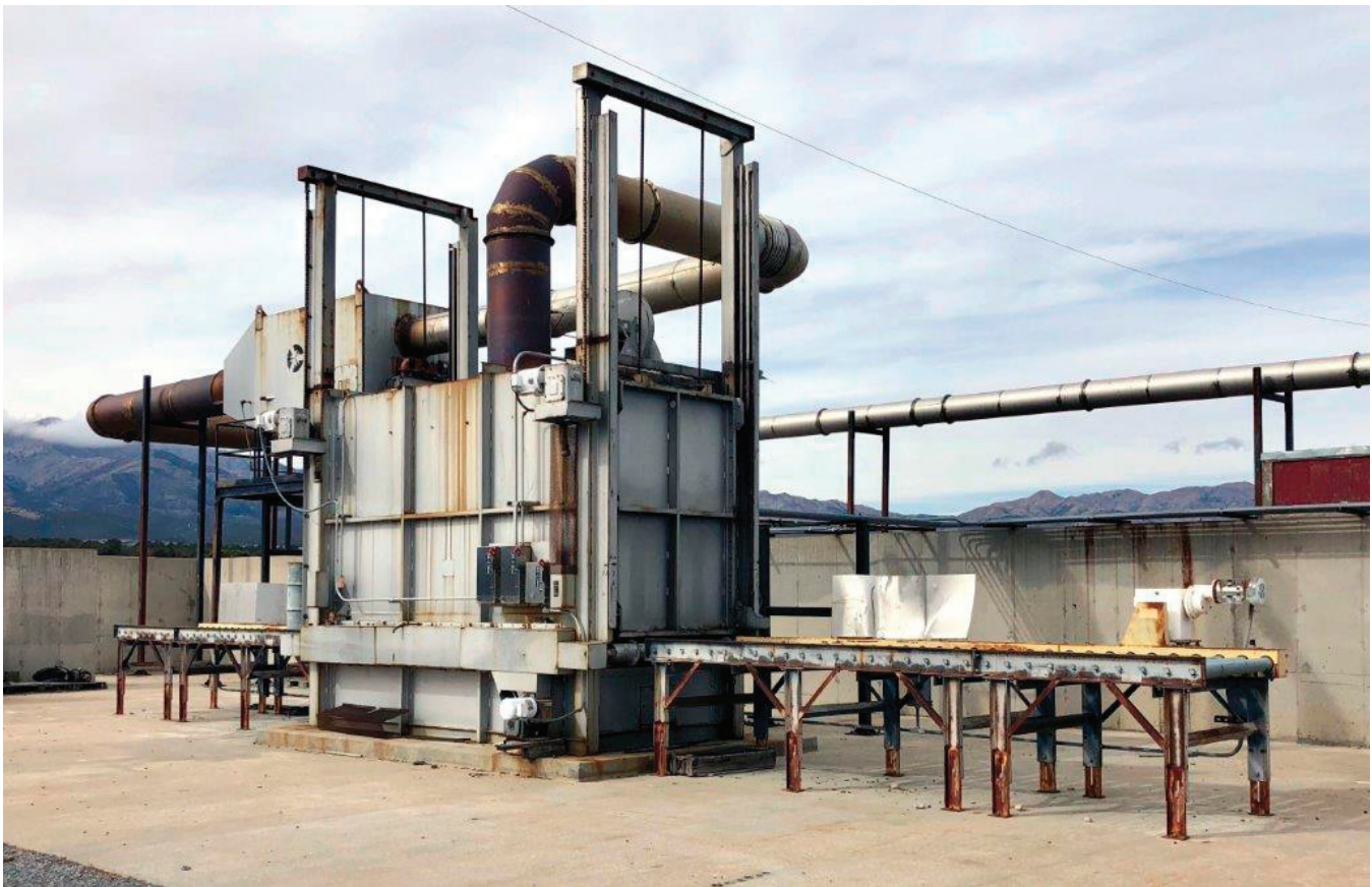
FIGURE 4.6 APE 2048 flashing furnace. SOURCE: J. McFassel, product director for demilitarization, PEO AMMO, and O. Hrycak, chief engineer, Office of the Product Director for Demilitarization, PEO AMMO, “Emerging Technologies Addressing Alternatives to Open Burn and Open Detonation,” presentation to the committee, August 22, 2017.
