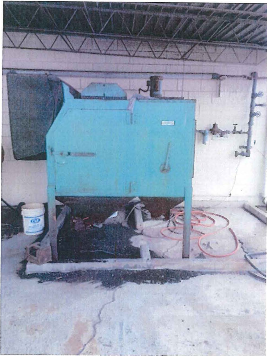
Picture 12: Holston Army Ammunition Plant – December 10, 2015 at 11:45 A.M. Release from the sand blasting unit outside the Paint Shop. Picture taken by Javier Garcia.
