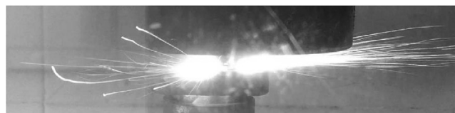
Fig. 20. Violent exothermic reaction of Al-PTFE during quasi-static compression [137].
