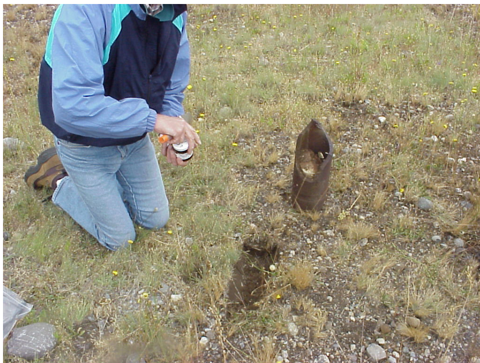
Figure 20. A 155-mm round that had broken open due to a low-order detonation
