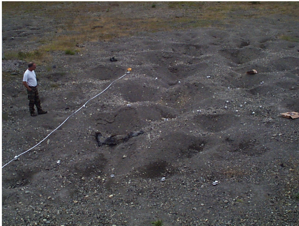
Figure 2. Hand grenade range at Fort Lewis. Tape extends perpendicular from launch area. Note sample jars in rows perpendicular to tape at 15, 20, and 25 m from launching areas
