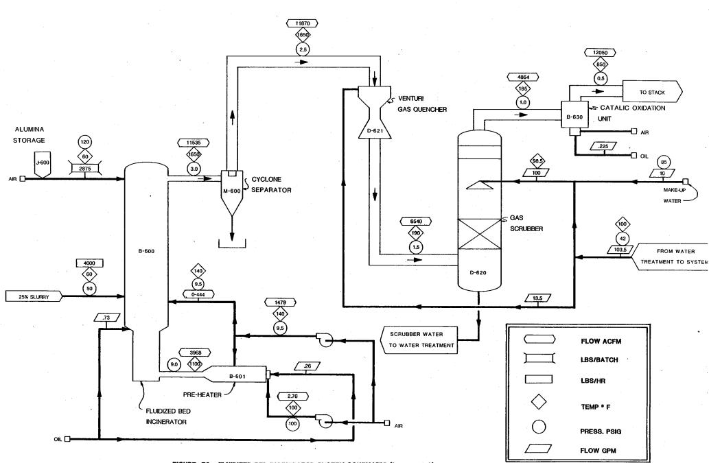
FIGURE E3 - FLUIDIZED BED INCINERATOR SYSTEM SCHEMATIC (Increment 2)
