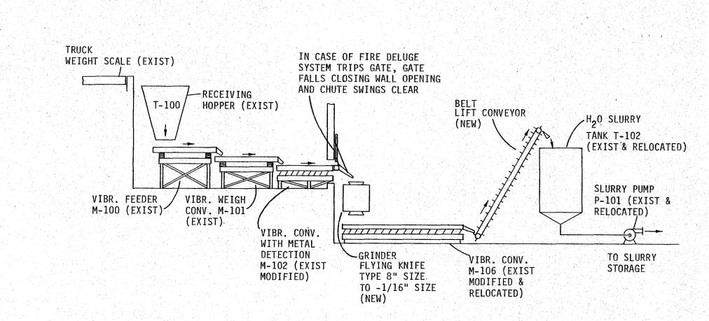
NOTE: THE COMPLETE SYSTEM IS TO HAVE A WATER SPRAY SYSTEM TO PREVENT TEMPERATURE RISE OF PROPELLANT.
