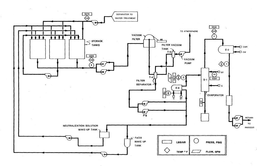
FIGURE E2 - WATER TREATMENT SYSTEM FOR WET AIR OXIDATION SYSTEM (Increment 1)
