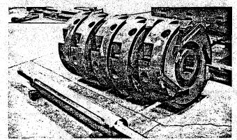
Heavy-duty rotor sections and shaft before assembly
