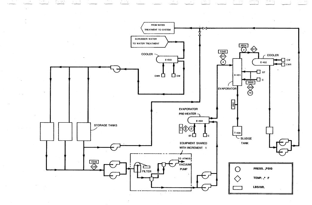
FIGURE E4 - WATER TREATMENT SYSTEM FOR FLUIDIZED BED INCINERATOR
