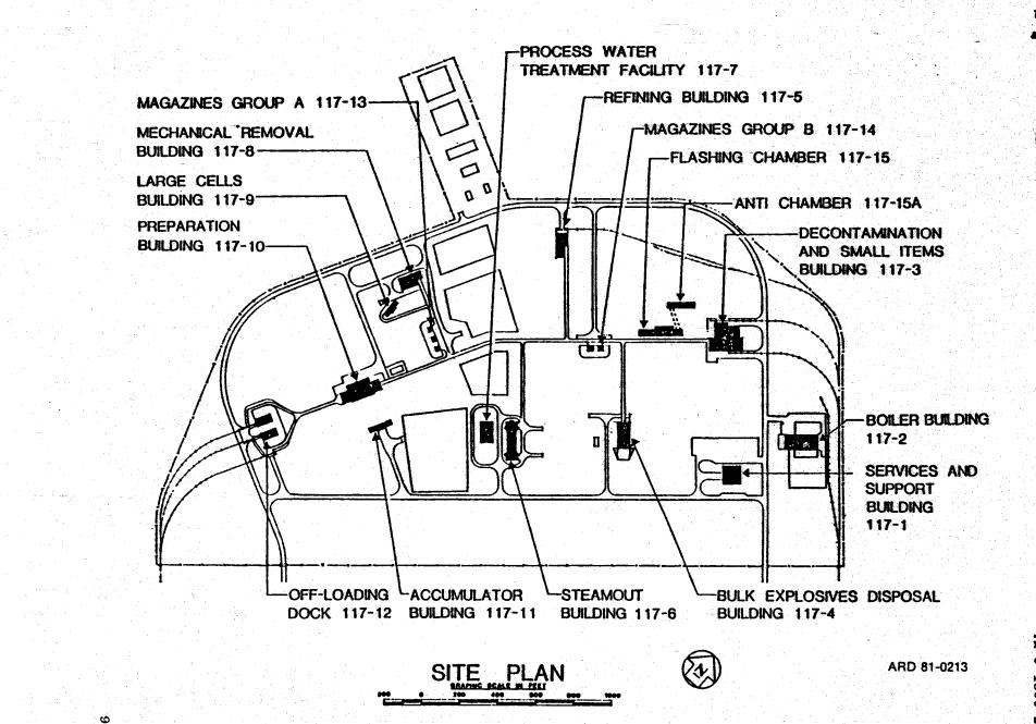
Figure 9-2. Site plan showing locations of all principal buildings, roads, and rail lines.
