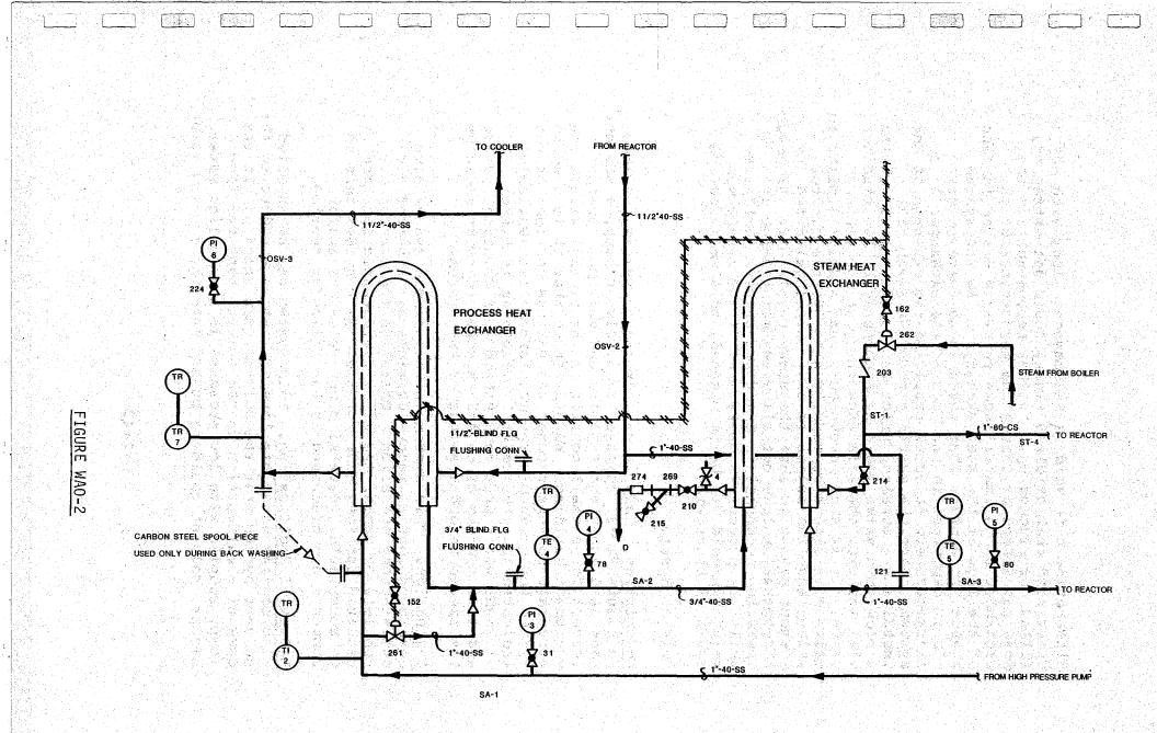
WET AIR OXIDATION EQUIPMENT - HEAT EXCHANGER FLOW DIAGRAM
