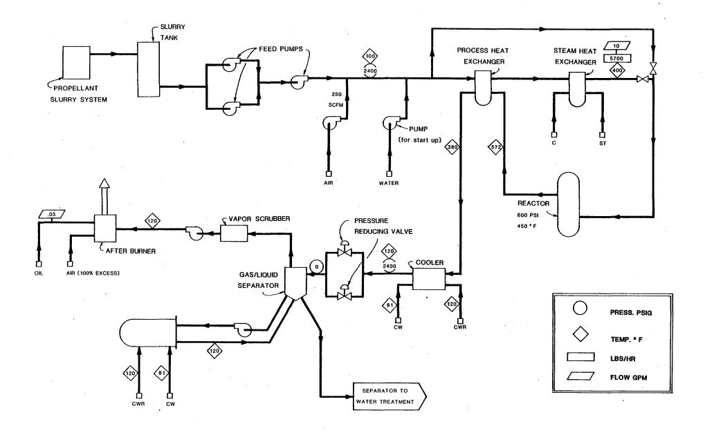
FIGURE E1 - WET AIR OXIDATION SYSTEM (Increment 1)
