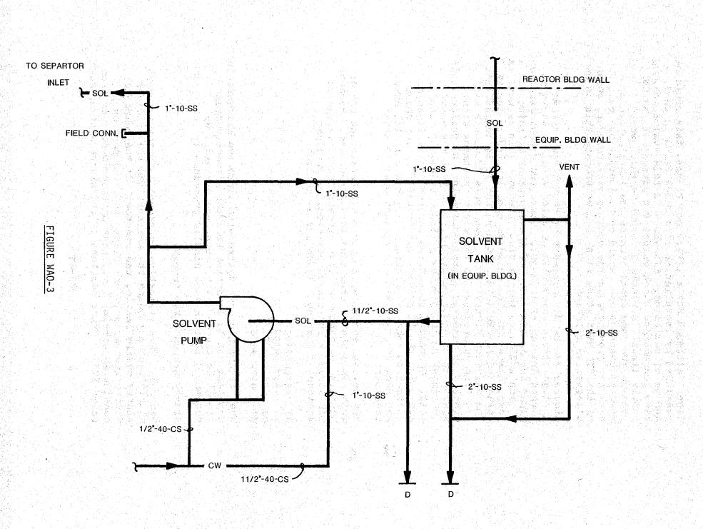
WET AIR OXIDATION EQUIPMENT - SOLVENT SYSTEM
