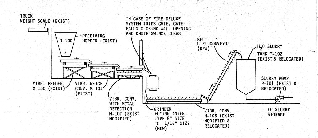
NOTE: THE COMPLETE SYSTEM IS TO HAVE A WATER SPRAY SYSTEM TO PREVENT TEMPERATURE RISE OF PROPELLANT.
