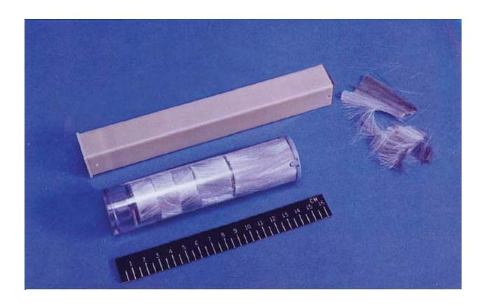
Figure 1. Radio frequency chaff cartridges (Air Force version RR-188/AL, top; Navy version RR-144/AL, bottom) and chaff fibers (right). Fibers of different lengths can be seen in the Navy operational version (clear cylinder). These lengths correspond to the frequency modes of the radar spectrum. In training, however, cartridges containing only 1.8 cm fibers are used (not shown).
